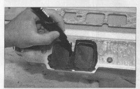
Then use a marking dye on the intake. A product called Dykem is used by professionals for this, and you can order it from most mail-order houses when you purchase a Standard Abrasives porting kit. We're cheap so we used a wide-tip felt-tip pen instead.
