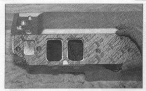
You must have a plan before breaking out the die grinder. Intake-port matching is one of the easier porting jobs to tackle, so that's what we did for this article. Select an intake gasket with intake-port openings that are the same size as the ports in the cylinder heads.
