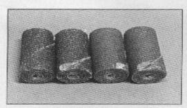
The lower the grit number, the more aggressive the sandpaper. The 40-grit rolls (the two on the left) should be used first to remove larger amounts of metal. Follow this with an 80-grit roll (right). These are used to create the basic shape. Tapered versions in both grits are included in the kits in addition to the straight ones shown to ease porting in tight areas.
