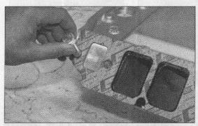
Position the gasket on the intake in a manner that you can repeat on both sides. We found that %-inch bolts fit perfectly in this Mr. Gasket big-block Chevrolet intake gasket (PN 110) and Edelbrock Victor 454-R intake (PN 2907). This is a very important step since matching the intake ports is worthless unless you can line up the heads, gaskets, and intake manifold once you're finished porting.
