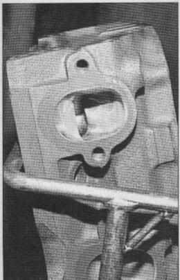
Instead of laying down the extra cash for a set of aluminum heads, consider porting the existing heads to increase the flow. Stock 460 heads have a large lobe (arrow) in all the exhaust ports that significantly hinder flow and rob the engine of horsepower. In the second photo, the lobe has been removed and the entire port has been smoothed and polished.
