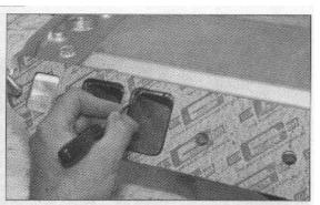
With the intake gasket in the correct position, use a scribe to scratch a line around each of the ports. This will be your guide or outline for your work. The scribe we used was from Harbor Freight and cost about \$1—they're available from most tool stores.
