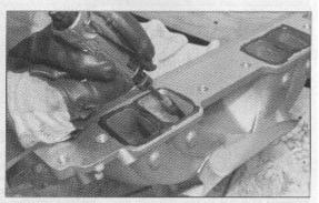
The corners can be a little difficult to shape with the large roll. We switched to a tapered 40-grit roll to rough in these areas. Try to keep the end of the mandrel and the chuck portion of the grinder from hitting the port as this will create a rough area you'll need to fix.
