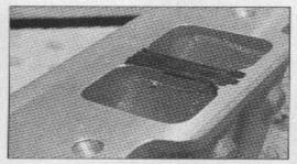
These are some of the big items you can clean up in the ports. Our goal with this intake wasn't to drastically alter the shape of the ports. Instead, we wanted to match the portoutlet size to the gasket (the cylinder heads were matched to the same gasket by a professional porter), and remove any obvious hindrance to flow.
