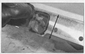
We began with a 40-grit roll in an area that needed a lot of material removed because proper control and finesse will take awhile to achieve. Keep the roll moving steadily (arrow) to avoid creating a dip. You want to remove material uniformly. At first, be only concerned with the end of the port (at the gasket): The rest will be blended in later.
