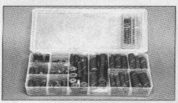
The Cartridge Roll kit comes with plenty of 60- to 120-grit rolls. This is a good supplemental or refill kit for the other porting kits. The rolls are smaller (%- to %-inch diameter) than those provided in the Standard kit. The smaller size is also easier to use in certain areas of an engine.
