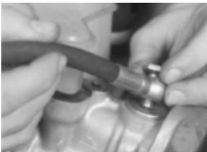
**P15-7** Disconnect the high-pressure hose from the pump.
