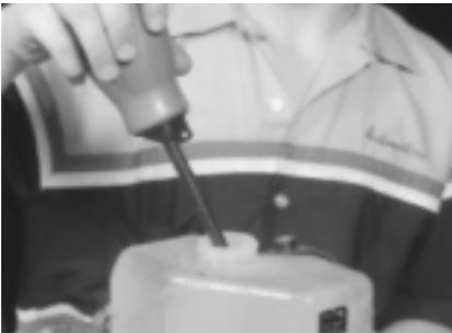
**P15-5** Use a clean syringe to remove about half of the brake fluid from the reservoir.
