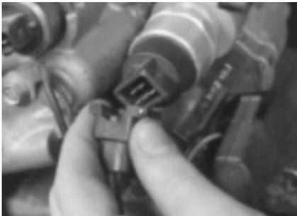
**P15-4** Disconnect the electrical connectors from the pressure switch and the motor.
