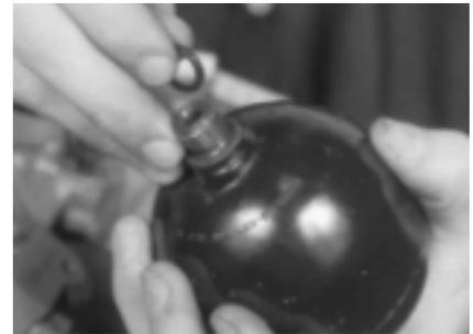
**P15-6** Unscrew the accumulator from the hydraulic module. Then remove the O-ring from the accumulator.
